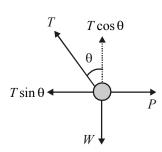
As the metal sphere is in equilibrium under the effect of the three forces therefore
